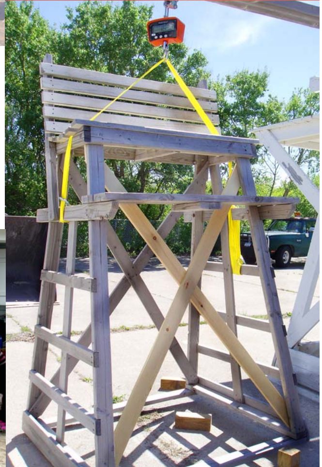
Left: In an attempt to lighten our wingstands and have a uniform construction, Bob Adler weighed numerous stands.
